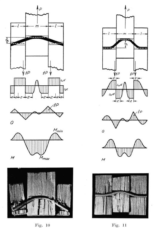
$$\begin{split} \frac{1}{2}\,P &= s_H\,dz \quad \text{and} \quad x = \frac{1}{2}\,(l-z)\,,\\ M_{max} &= \frac{\pi}{32}\,s_B\,d^3 = \frac{1}{2}\,Pz - s_H\,dx^2 = s_H\,dz^2 - \frac{1}{4}\,s_H\,d\,(l-z)^2\\ z &= \frac{l}{3}\left(\sqrt{4 + \frac{3\,\pi}{8}\,\frac{s_B}{s_H}\frac{d^2}{l^2}} - 1\right) \end{split}$$
