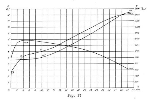
than with the normally tensioned bolt. The ultimate load  $P_{max}$  was the same for all the tests, i.e. unaffected by the initial tension of the bolts, which is also expressed in (7).
