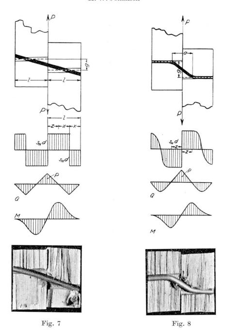
If the dowel is not sufficiently stiff it will be bent as shown in Fig. 8. In bending, the moment is  $\frac{\pi}{32} s_B d^3$  and the transverse load 0; between the bends the crushing is so heavy that the pressure is practically  $s_H d$ . About the pressure outside the bends nothing definite is known, nor is this of any consequence, as the static conditions are formulated only for the length of dowel between the bends.
