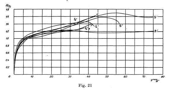
ding and rupture and suitable small slips at the working load. For dowels we thus get the slip
