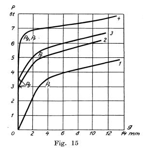
ionless bolt  $P_g$  lies, of course, at zero, as the curve also shows. With the greatest bolt tension,  $P_g$  and  $P_F$  are less marked and coincide. When the bolt is tightened till the threads are mutilated,  $P_g$  and  $P_F$  are placed but little higher
