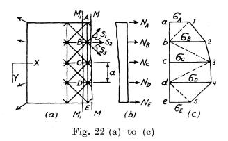
The edge stress, such as  $\sigma_A$ , cannot in general be found by Eq. (5) without violating statics, since the centre of the triangle ab 1, into which the concentration  $N_A$  is converted, does not coincide with the point A. Three cases should be distinguished in this connection:
