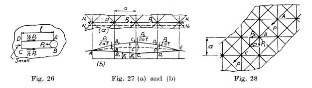
rated from the plate, and its equilibrium is considered. If the length of the strip l is sufficiently great, the stress at the end DC is small, and the average shearing stresses on the planes AD and CB become  $\pm \frac{P_r}{2 l t}$ , as follows from statics and symmetry. With a single rivet load acting on the plate there seems to be
