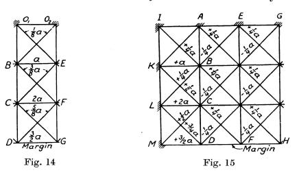
7. Rotation and shear combined, Fig. 15. Here the lines AD, EF and GH are rotated separately through equal angles in the same direction about the points A, E and F respectively.
