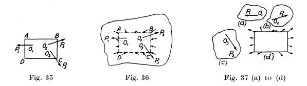
let the stresses existing in this infinite plate along the obliterated now former boundaries be as shown in Fig. 36, these stresses representing the action of the outer part of the plate on the inner part ABCD. The state of stress in the original finite plate (Fig. 35) may evidently be considered as a combination of the following four states, shown separately in Fig. 37 (a) to (d).
