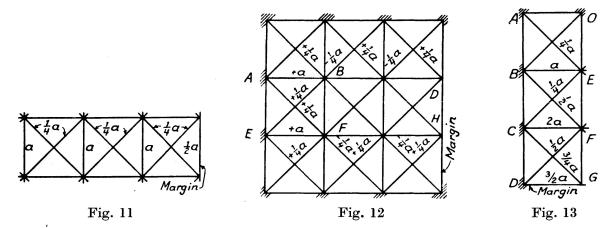
6. Rotation about an exterior joint, Fig. 13. The right hand part of the framework is rotated about the joint 0 in such a manner that the joint E moves horizontally a units to the right. The joints F and G then move 2a and 3a units respectively, which explains the stresses produced.
