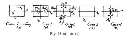
of Fig. 17. This is illustrated in Fig. 18 (a) to (e), from which it may be seen that one of the component cases, namely  $A_xS_y$ , is missing. In the three remaining cases forces  $\frac{1}{4}P$  and  $\frac{1}{4}Q$  are assumed to be applied to their respective quadrants. A more restricted special case, in which a load is applied at the centre of the framework, is shown in Fig. 19. With this loading three of the four component cases are missing.
