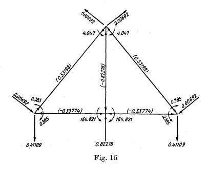
Fig. 15 shows the end moments of the frame together with the corresponding panel loads. The axial forces produced in the different members are written in brackets. The changes in lengths due to these axial forces are:
