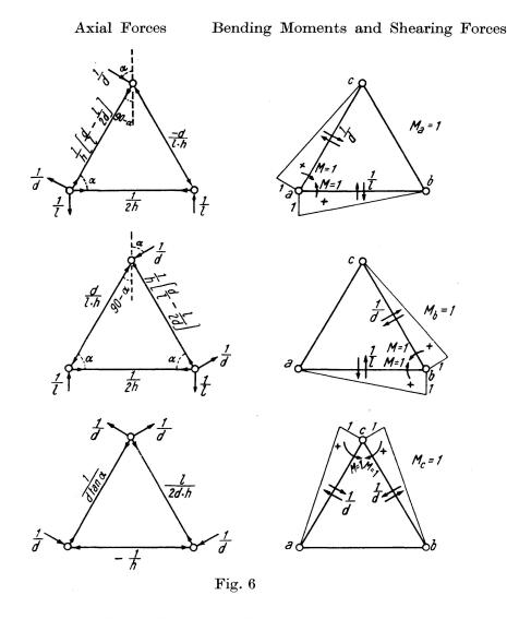
Consider now the effect of a non-uniform change in the temperature of the main system. Let the side ab expand a distance  $\Delta = a \cdot t \cdot l$ , due to a rise of  $t^0$  in its temperature relative to the other two members. These latter experience no change in length.
