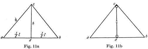
The bending moments produced at the rigid connections are calculated first by the method of work, and then by the method of joint rotations. In the latter case, the joint displacements of the rigid frame are taken from the displacement diagram of an equivalent frame with pinned connections, corresponding to what is generally done in practice.
