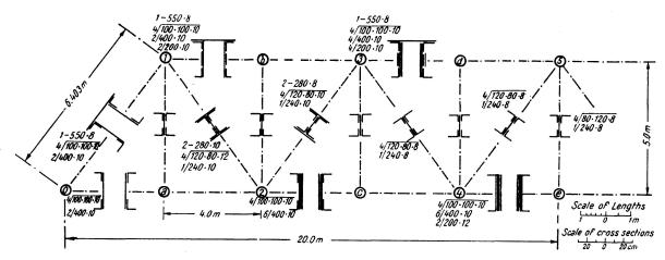
Fig. 16. Main Girder of a Single Track Railway Bridge designed according to Swiss Specifications
