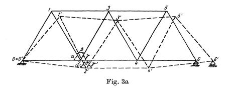
The members are not shifted parallel to themselves as in the case of a uniform change of temperature. On the contrary, they will be rotated and their slope angles changed. However, no stresses are produced in the members as long as the truss is provided with pinned connections and is statically determinate. The pinned connections allow every member to rotate freely about its end hinges, without any constraint.
