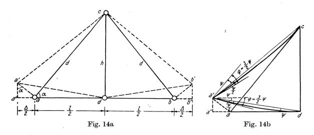
Keeping the direction of the central hanger unchanged, the change in the temperature of the lower chord causes a relative displacement of the two joints
