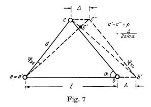
Further, since the frame is symmetrical, the rotations  $\psi_{ac}$  and  $\psi_{bc}$  of the system lines ac and bc must be equal and opposite. On the other hand, the system line ab will not rotate at all so that  $\psi_{ab} = 0$ .
