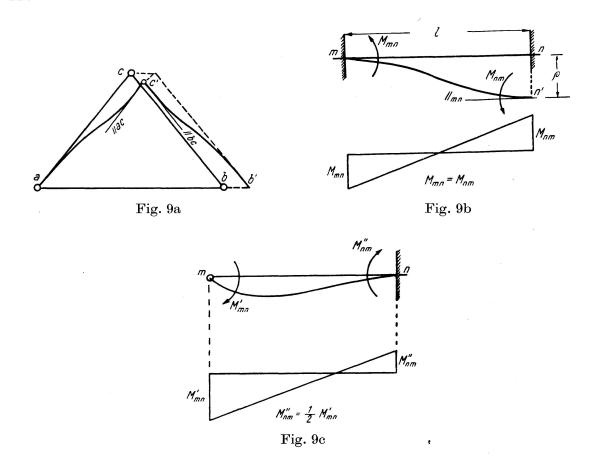
Let the end n, for example, of the fixed member mn, fig. 9b, deflect a distance  $\rho$  normal to the original direction of the member. The corresponding end moments are:  $M_{mn} = M_{nm} = -3 \ N \cdot \psi = -\frac{6 \ E \ I \ \rho}{l^2}$  where I = moment of inertia, l = length, and N = stiffness of the member mn. The negative sign denotes that, for a clockwise rotation of the member mn, both  $M_{mn}$  and  $M_{nm}$  will be counter-clockwise.
