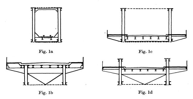
The change in the temperature of the truss may also be non-uniform. This is for example the case for a through bridge with side-walks, fig. 1c, which shelter the lower chord members from the direct heat of the sun or a direct cold wind. Also in the case of a deck bridge with upper chord members projecting above the floor, fig. 1d, the upper chord will be exposed to the direct sun beams, while the web members and the lower chord will be sheltered by the side walks and the floor.
