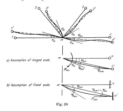
Consider now a group of members to be rigidly connected together at a certain joint m, fig. 20. Assume further that the ends 1, 2, 3, . . and n of the members are displaced, relative to the common joint m. This case represents obviously the condition of a similar joint in a truss.
