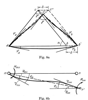
Since the angles between the system lines are changed, the members of the rigid frame must bend so as to keep the angles between the end tangents at the connections unaltered, fig. 8a. In this way the joints will prescribe angular
