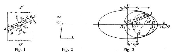
If e. g. the shearing energy was assumed to be determinant for the appearance of plastic deformations, so that the hypothesis of Huber-von Mises-Hencky is valid, and in this connection, since there is no preference for any plane, that the material behaves quasi-isotropically under the plastic deformation, then it appeared that the state of stress established itself prior to the yielding of the section in such a manner that a maximum resistance is obtained.
