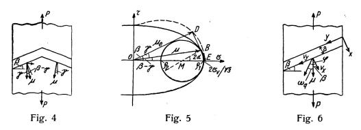
That this is indeed the case, results from the fact that during the yielding of a weakened strip according to fig. 1, the lower part of the plate moves with respect to the upper part in a direction which we have termed the direction of yielding, and which embraces an angle  $\omega_q$  with the axis of the plate (fig. 6). The displacement  $\nu_x$  of the lower portion of the plate with respect to the upper portion is namely, also in connection with (6):
