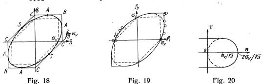
The stress required for the appearance of the first yield lines is the upper yield point; the stress to which the yield stress decreases on its further spreading, whereby the contraction is practically not impeded any longer, is the lower yield point. The upper yield point and probably also the elastic limit is consequently determined by the limit figures for local yielding, the lower yield point consequently by those for unimpeded yielding.
