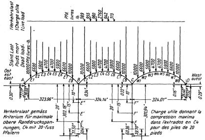
Live load based on criterion for maximum compression of extrados, C4, with 20-ft. piers
