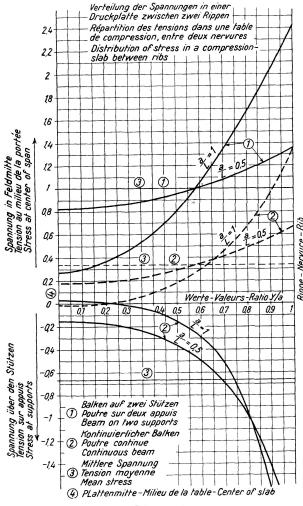
Abstand zweier Rippen 2a. Distance entre nervures 2a. Distance between ribs 2a.
