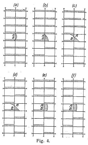
The design of a stanchion length, therefore, resolves itself into two steps, 1. the determination of the end reactions applied to the member by that arrangement of load on the structure which produces the worst conditions in the member, and 2. the estimate of the maximum stress developed in the member by those reactions, enabling the suitability of the member to be judged.
