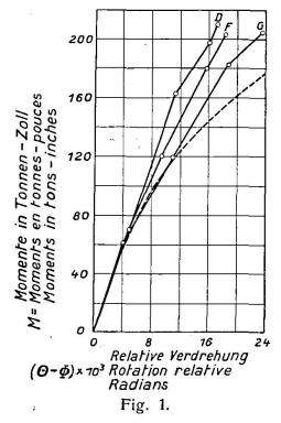
curves between M, the moment transmitted, and  $(\Theta - \Phi)$ , the relative rotation of the members joined by three similar connections consisting of  $4^{in} \times 4^{in} \times \frac{1}{2}^{in}$  flange cleats  $8^{in}$  long and  $4^{in} \times 4^{in} \times \frac{1}{2}^{in}$  web cleats  $10^{in}$  long are plotted together with the lower limit curve, shown by the broken line, deduced from the laboratory tests.
