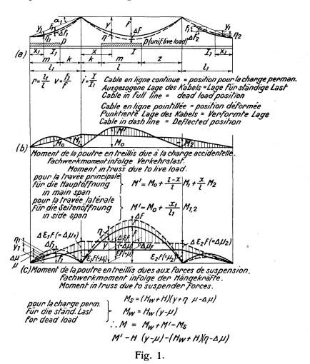
In consequence of the deflections  $\eta$  (see Figs. 1 a and 1 c), the cable ordinate y increases to  $(y + \eta)$ , and  $\mu$  increases to  $(\mu + \Delta \mu)$ . Accordingly the bending moment M at any section, as given by Eq. (2), is relieved by the additional amount:
