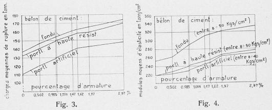
Charges moyennes de rupture en tonnes — Mittlere Bruchlasten in Tonnen — Average loads of rupture in tons.
