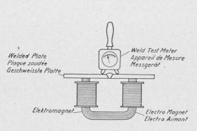
Ratio of Weld Reading to Plate Reading—
