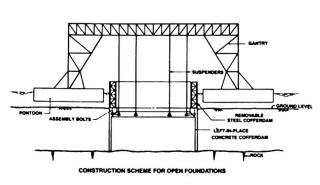
Fig.6 Detail of floating gantry with cofferdam assembly
