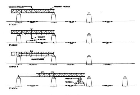
Fig.16 Sequence of assembly of superstructure
