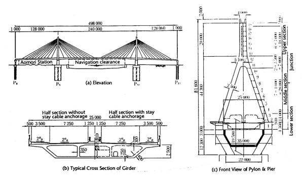
Fig. 2 General View of the Cable-Stayed Bridge
