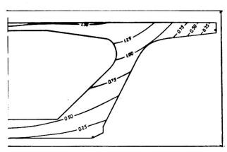
Fig. 3 Distribution of glued joint thickness along its surface (isolines values are ji-ven in mm)
