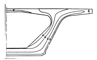
Fig.1 Temperature field in the middle section of a segment-mat-rix (isolines values are given in °C)
