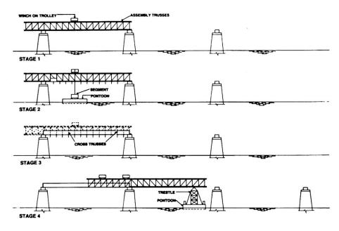
Fig.16 Sequence of assembly of superstructure
