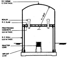
Fig. 1 Cross Section
