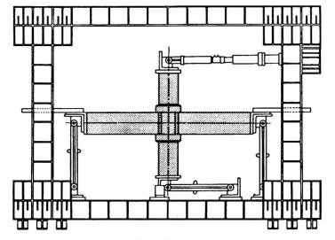
Fig. 9 Testing of column-to-beam joint
