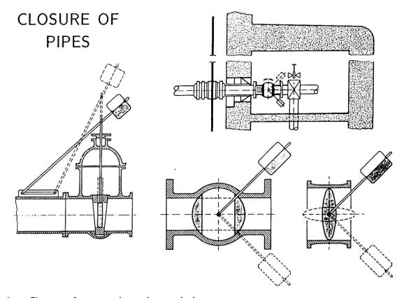
Figure 4: Closure of penetrating tubes and pipes
