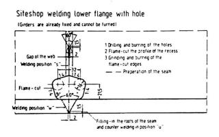
With joints of the site shop, conditions should be avoided in predicaments, if possible. For this reason a welding on one side in the form of V-butt welds for flange welds is realized (figs. 5 and 6).
