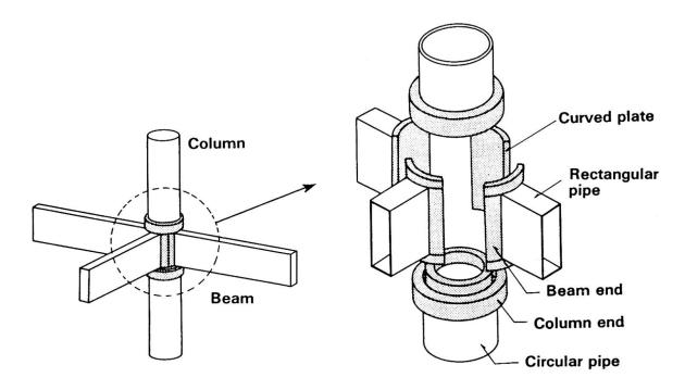
Fig. 3 Column-to-beam joint
