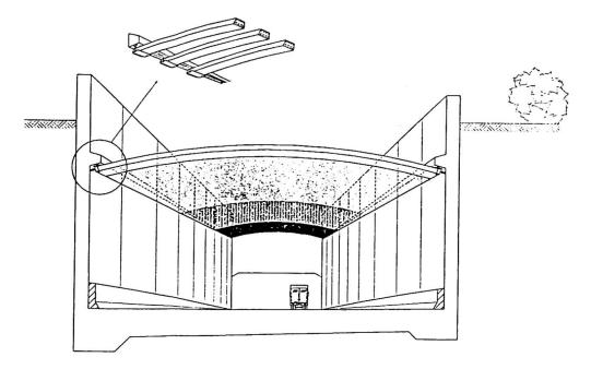
fig. 9: Perspective view of a tunnel daylight screen
