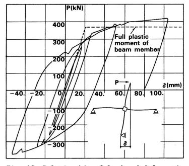
Fig. 10 Relationship of load and deformation
