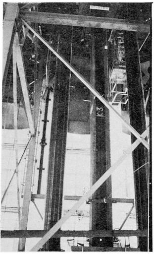
Fig. 3 shows the test specimen with a flange thickness of 97 mm and a length of 8,0 m in the 50 MN-testing machine of the Versuchsanstalt für Stahl, Holz und Steine.
