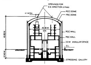
Fig.6 Section of Kaiga Containment
