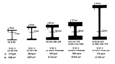
The load bearing behavior of butt welded, thick-walled beams under static and fatigue load has also been investigated in Karlsruhe. Fig. 7 shows the dimensions of the sections in the tests.
