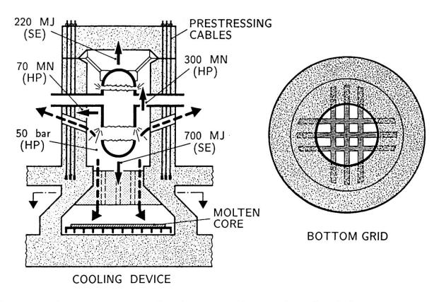
Figure 3: Reactor pressure vessel environment and core-melt cooling device
