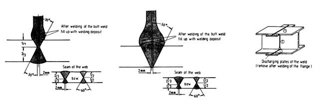
Fig. 6 Butt welded connections without holes on beams
