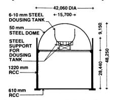
Fig.1 RAPP Dome - Original proposal in Steel
