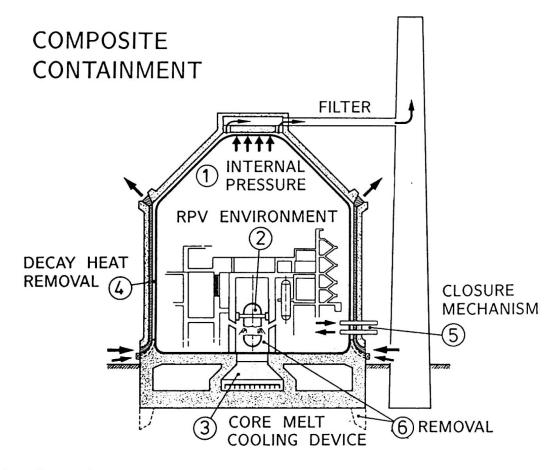
Figure 1: Composite containment for a pressurized water reactor
