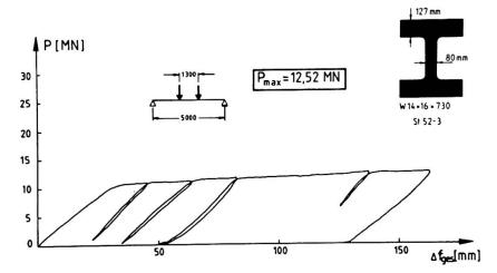
Fig. 12 Load deformation diagram for thick-walled rolled beams
