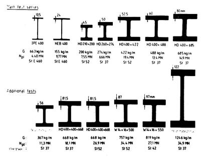
Large size rolled sections have already passed their test for the application as compression members. For the classification in buckling stress curves of Eurocode 3 [1] corresponding investigations have been made in Karlsruhe with the sections (flange thicknesses up to 122 mm) illustrated in fig. 2 [2].
