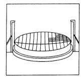
Finally, thin glass mirrors are bonded onto the front membrane.
