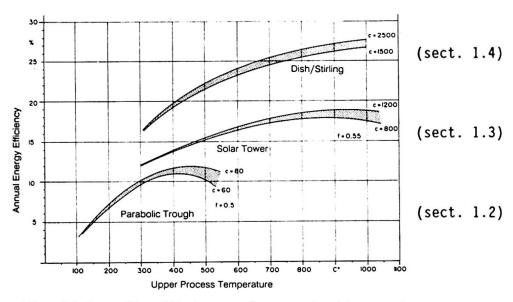
Fig. 11 Overall efficiency of concentrating systems
