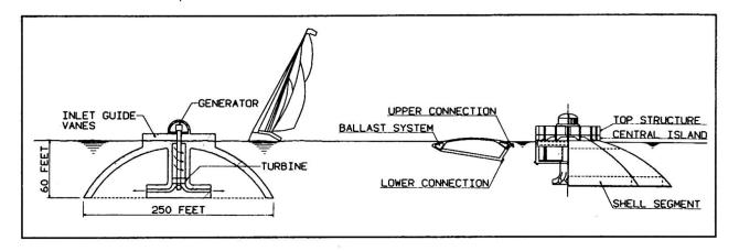
Fig. 7 Dam atoll in place and under construction
