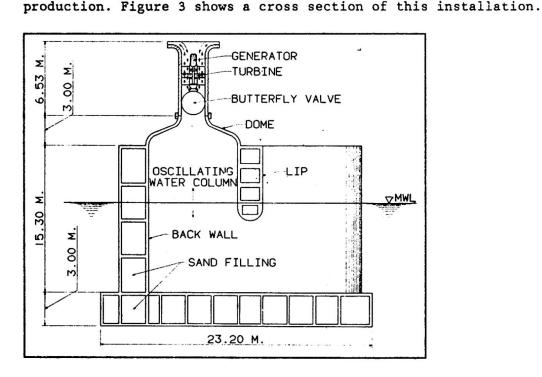
Fig. 3 Experimental wave energy generator offshore Tamil Nadu
