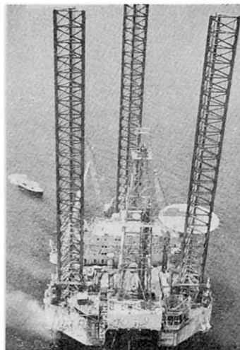
Fig. 6 Self-raising platform, "TRIGONE"
