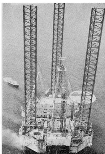
Fig. 6 Self-raising platform, "TRIGONE"
