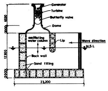
Fig.1.a Cross section of wave power plant
