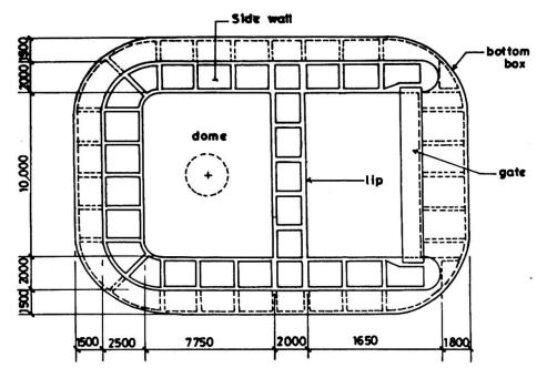
Fig.1.b Cross sectional plan of Caisson
