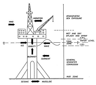
Fig. 2 Major platform loads and corrosion zones.
