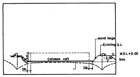
Fig.3.a Construction of bottom box and bund
