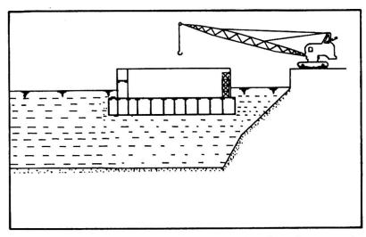
Fig.3.b Construction in floating mode
