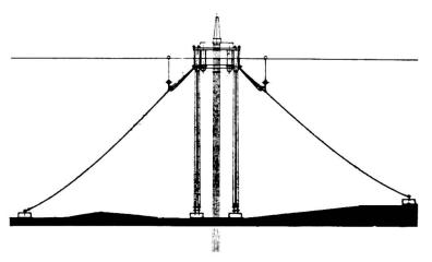
Fig. 21 Anchroring system, consisting of vertical and oblique cables.
