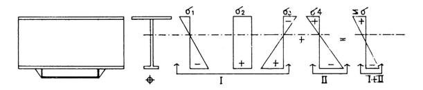
STAGE - I - FROM DEAD LOAD + PRESTRESSING STAGE- II - FROM LIVE LOAD INCLUDING IMPACT
