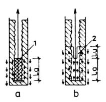
Fig 4. Eficiency of tie-bar with prebulb a.tie-bar without prebulb; b.tie-bar with prebulb 1.area with cracks ;2.prebulb with a washer effect
