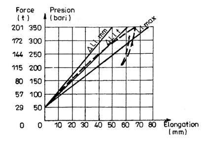
Fig.7 Diagramme of the tie-bar tensioning
