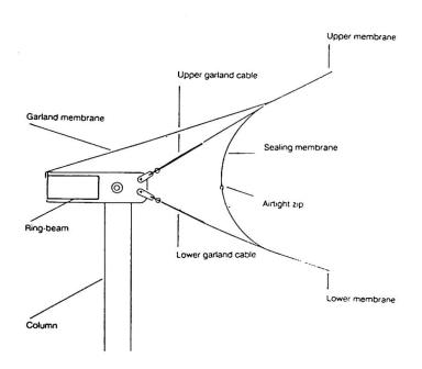
Fig. 9 Arena Nimes Vertical section at the perimeter of the cushion.
