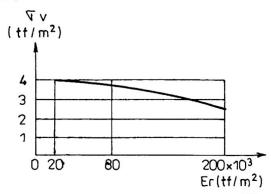
Fig.6-Variation of normal unitary effort  $\nabla v$  at the contact between rock and tie bar, at the upper side of the bulb, according to the size of the elasticity modulus of the rock Er
