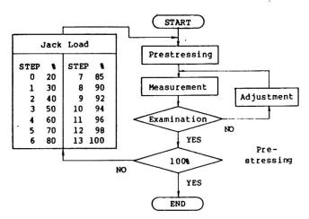
Fig. 9 Flowchart of Prestressing and Measurement
