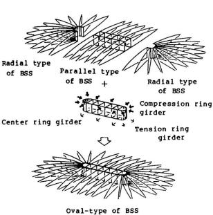
Fig. 3 Structural System
