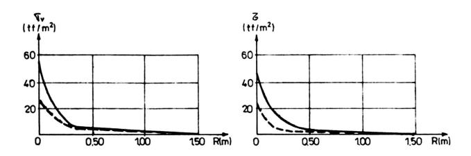
Fig.5 Diagramme of normal and tangential unitary efforts at the level of the contact area between bulb and prebulb
