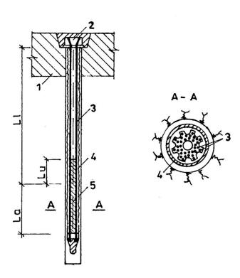
Fig.3 Anchoring cross-bar for the dry dock bottom
