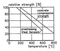
Fig. 5 Temperature distribution over Fig. 6 Temperature dependency of conthe shell thickness after 10 hrs [6]. crete and steel strength (after [8].
