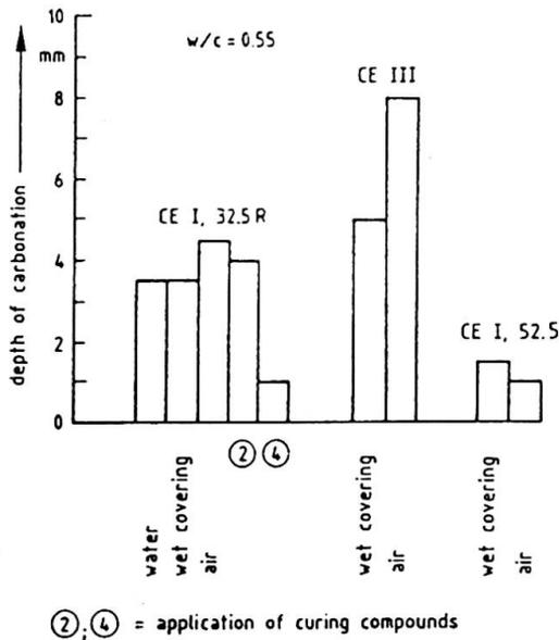
Fig. 3: Effect of various curing methods on the depth of carbonation at a concrete age of 6 months [5]
