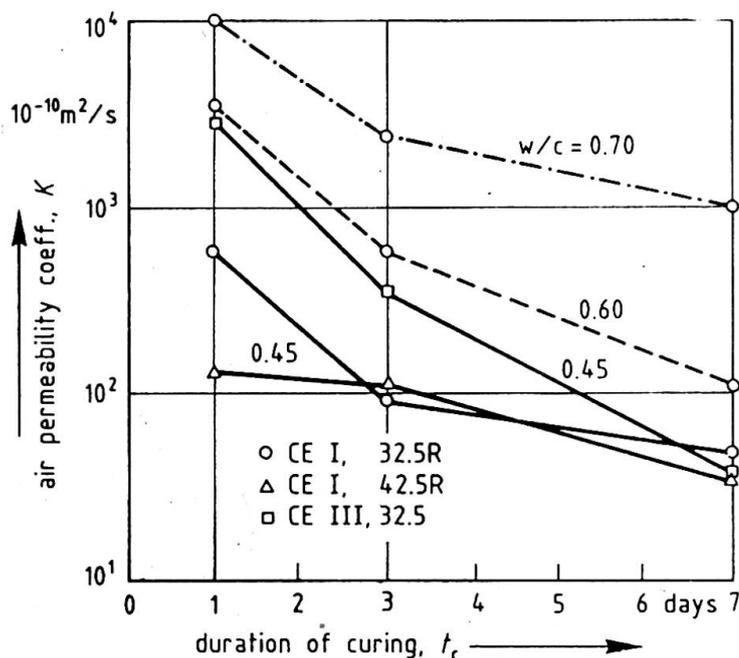
Fig. 2: Effect of the duration of curing on the air permeability coefficient of various concretes [3]
