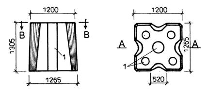
Fig.5 Concrete block (G=150 KN) acted biollogically 1-cylindric emptys
