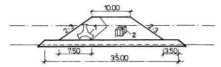
Fig.4 Breakwater-cross section 1-stabilopod 200 KN; 2-bioactiv block 150 KN
