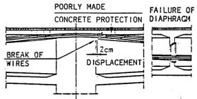
Fig. 12 - POORLY MADE CONCRETE PROTECTION
