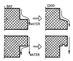
Fig. 2 - SHAPE OF CONCRETE SURFACES
