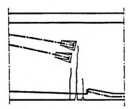
Fig. 14 - TENDONS ANCHORING WITHOUT OVERLAPPING
