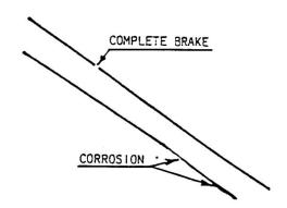
Fig. 9 - VERY CORRODED PRESTRESSING WIRES
