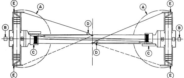
A Tower Crane B Personnel Hoist C 5 Tonne Winch D 10 Tonne Pulley F Portal Beam
