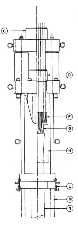
Fig. 3 3F/Vemac 600 Tonne Cable Stressing System - Jack and Stool
