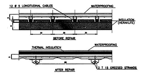
Fig.2 Section through shell
