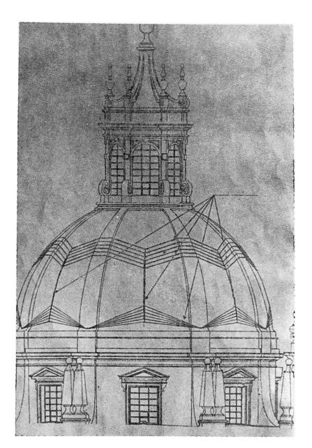
Pic.31: Prestressed cables for the reinforcement of the dome
