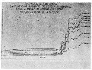
Pic.34: Monitoring of the phases of prestressing
