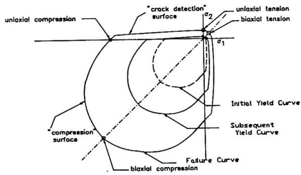
Fig. 2 Concrete Failure Surfaces In Plane Stress
