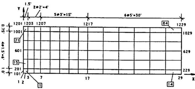
FIG. 9. Finite Element Model ( 1 in = 25.4 mm )
