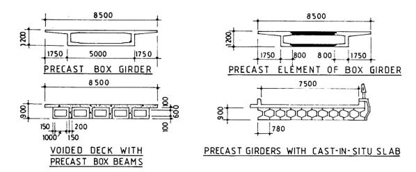
Fig.1: The various alternatives for the viaduct spans
