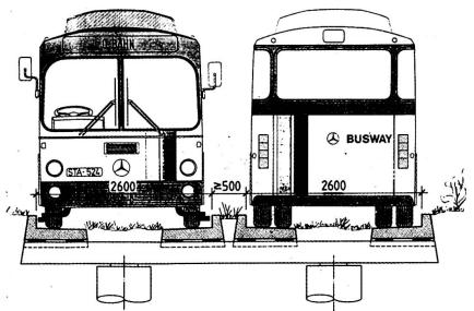
Fig. 1 Cross section of double lane
