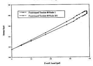
Stress of Tendon in X-direction (1 ksi = 6,895.0 kPa; 1 psf = 47.88 Pa) Fig. 13
