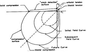
Fig. 2 Concrete Fallure Surfaces In Plane Stress
