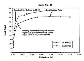
FIG. 4. Deflection at Node 1 in Z-direction (1 in = 25.4 mm; 1 kip = 4.48 kN)
