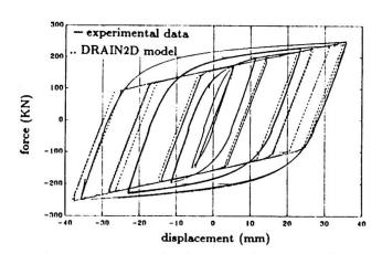
Fig. 2 Hysteretic loops of a test beam
