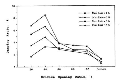
Fig. 4 Variation of damping ratio with orifice opening and mass ratio for 100% tuning
