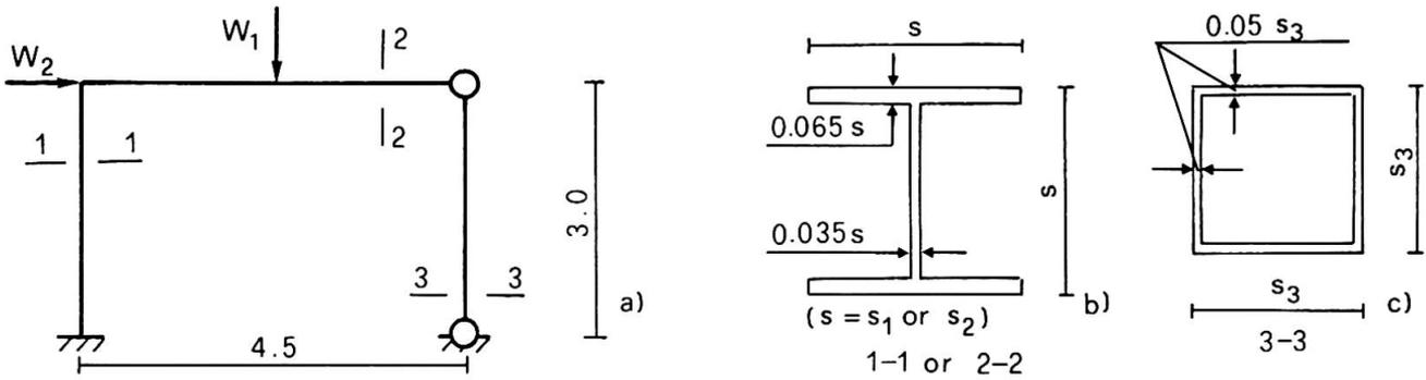
FIGURE 1 (from Ref. [2]) - Example design problem (lengths in meters). Economical parameters: total benefit in case of full success  $B^0=3000$ ; loss for total failure  $H_f=750$  or  $1500$ ; loss of excessive deformation  $H_d=3$  or  $15$ ; interest rate  $\gamma=5\%$  or  $15\%$ . Monetary unit: 1 kg of steel for  $B^0$  and  $U$ ; 1 t of steel for  $H_f$  and  $H_d$ . Loads: mean values  $W_1=2.8$  t;  $W_2=0.7$  t; coeff. of variation  $c_{W1}=0.1$ ;  $c_{W2}=0.2$ .
