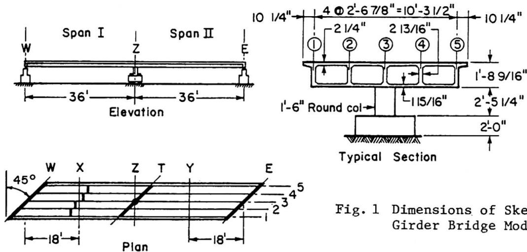
Fig. 1 Dimensions of Skew Box Girder Bridge Model
