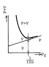
If we call n the ratio of the total damage caused by the collapse of one element and the price P of that element, then the sum of the price P and the fictitious insurance premium V shows a minimum for approximately
