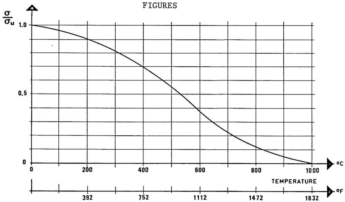
Figure 1 : Chart for calculation of critical temperature.
