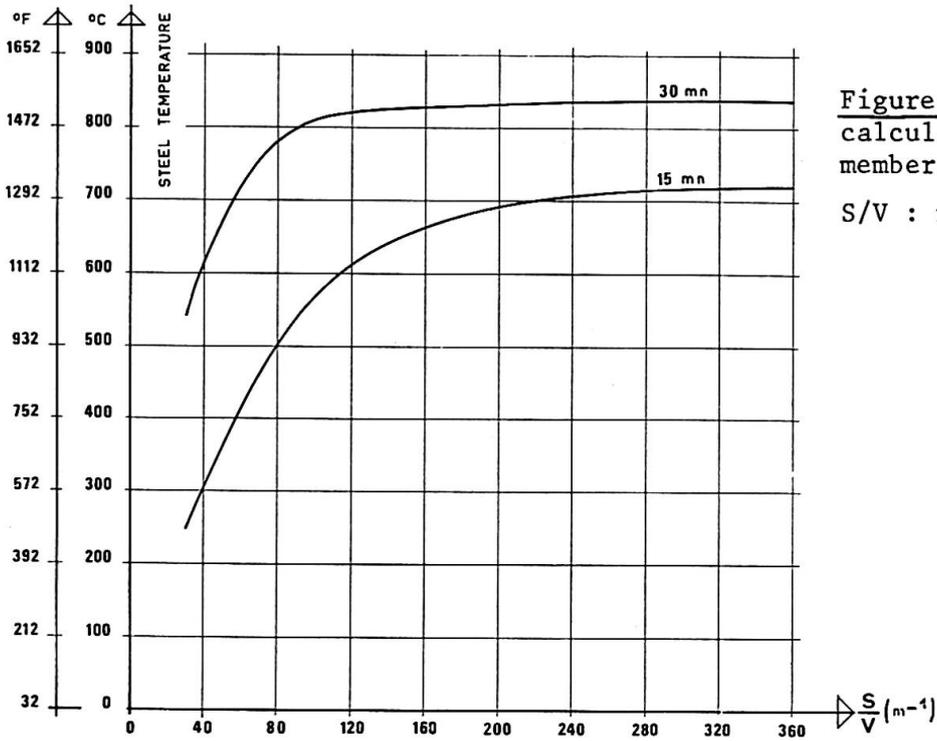
Figure 3 : Chart for heating calculation of non-protected member.
