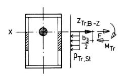
Fig. 4 Ultimate load stress distribution
