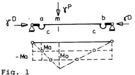
in fig. 1. The bending moment at position a for the given loads yP (lateral) and yD (axial) is to be checked with respect to the ultimate bending capacity of the connectors (c)
