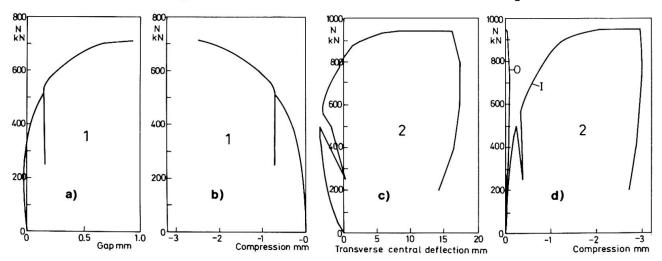
Fig. 6 a) Gap at outer side 0 and b) local compression at inner side I. Test no 1. c) Central deflection and d) local compression at inner side I and outer side 0. Test no 2
