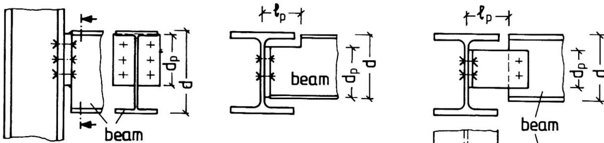
Fig. 1 Typical connections in building-structures
