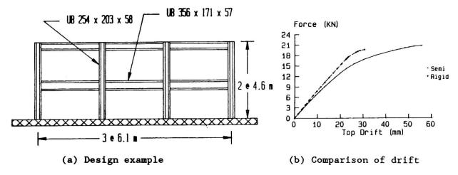
Figure 5 - Design example and comparison of drift for rigid and semi-rigid.
