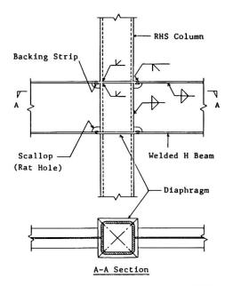
Fig.1 Wide flange beam-to-RHS column connection
