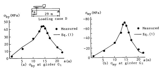
Fig. 10 Comparisons between the values by Eq. (1) and the measured ones
