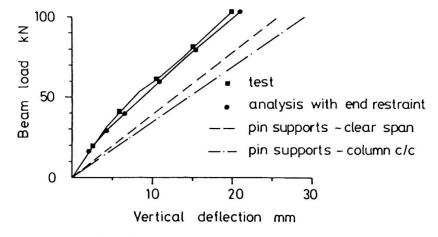
Fig. 5 Load Deflection Response of a Beam in Frame 1
