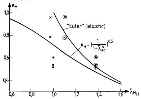
Fig. 2 Notched ends, evaluation of test results
