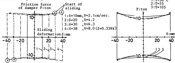
Fig. 3 Effects of Vibration Speed
