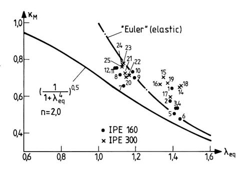
Fig. 3 Evaluation of test-results using assumption E3 - connection with end-plates
