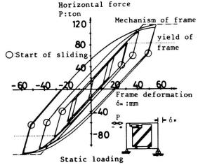
Fig. 8 Test Frame Restoring Force Characteristics
