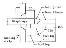
$\frac{\texttt{Fig.6}}{\texttt{connection}} \ \, \text{Detail of scalloped}$
