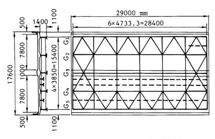
Fig. 2 General view of plate girder bridge
