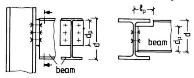
Fig. 1 Typical connections in building-structures To clarify the influence of the structural details of the conncetions tests were carried out at the Technical University of Berlin, reported by Lindner/Schulze (1985), [1], [2].
