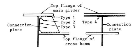
Fig.1 Fatigue cracks at cross beam connection
