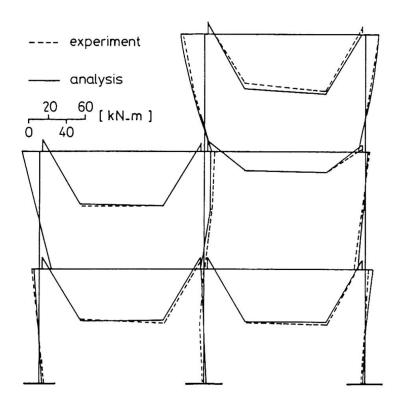
Fig. 2 Comparison of Measured Bending Moments and SERVAR Predictions Under
