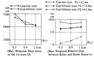
Fig. 9 Effect of Initial Gap Amount (δ<sub>G</sub>)
