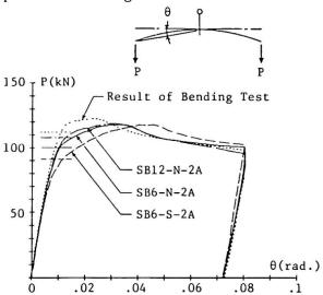
Fig.8 Simple beam with two axes of symmetry
