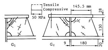
Fig. 5 Principal membrane stresses of connection plates
