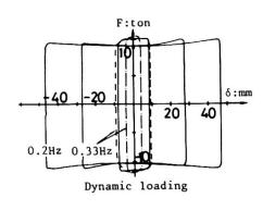
Fig. 10 Test Frame Restoring Force Characteristics
