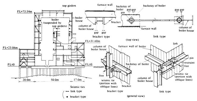
Fig. 1 Section of Boiler House (Takehara Thermal Power Station Unit No. 3)
