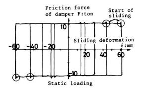
Fig. 9 Damper Characteristics
