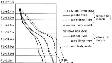
0.0 2.0 4.0 6.0 (x10<sup>3</sup> ton) \* base shear coefficient Fig. 6 Distribution of Max. Response Shear
