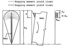
Beam with a single axis of symmetry
