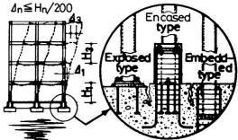
Fig.1 Three conventional type column bases
