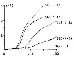
Fig. 10 Axial strain of tensile flange
