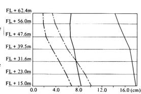
Fig. 7 Max. Response Relative Disp. between Boiler and Boiler House
