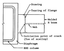
Fig.11 Tearing of tensile flange
