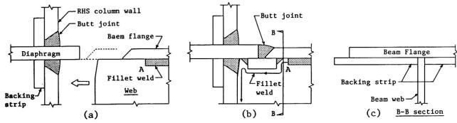
Fig. 7 Welding process of nonscalloped connection
