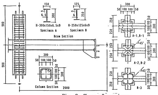
Fig. 2 Shape of specimens
