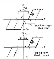
Fig. 5 Hystereses Models of Seismic Ties
