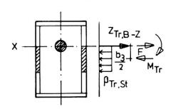
Fig. 4 Ultimate load stress distribution
