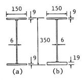
Fig.5 Beam section
