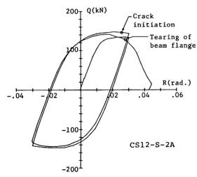
Fig.12 Q-R relation of cruciform subassemblage (with scallop)
