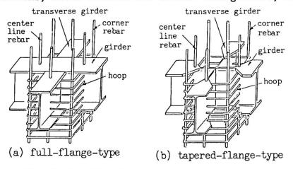
Fig. 1 Details of joint panels
