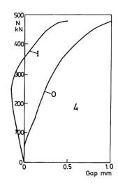
Fig. 7 Gap at the inner and outer side of the intersection between the connector and the member.
