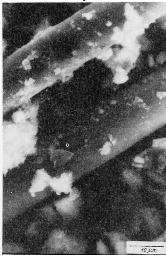
Fig.5 SEM of ESAP fibres in the cement matrix /360 days, water curing, fibres: 4.4%/
