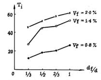
Fig. 7 Tougthness Index of SFRC as a Function of Fibre Content
