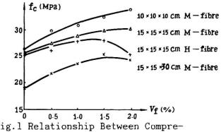
Fig.1 Relationship Between Compresive Strength of SFRC and Fibre Content
