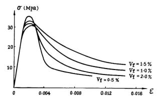
Fig. 5 Stress-Strain Curves in Compression for SFRC
