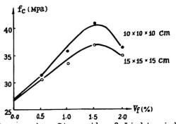
Fig.9 Compresive Strength of Lightweight Concrete Improved by Addition of Steel Fibres
