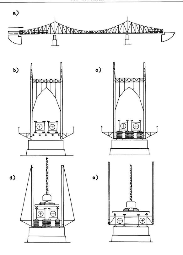
Fig. I The method of reconstruction of the metal superstructure of the Volga River Bridge in Kalinin: a,b- moving on blocks of the new superstructure; c- lowering of the moved on blocks onto the cades disposed on the permanent supports; d- cuttind of lattice trusses into blocks and dismountind them; e- moving apart the blocks of the new superstructure and erection of lattice truss assemblies along the front of the new superstructure and their egaging.
