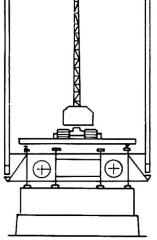
Fig. I The method of reconstruction of the metal superstructure of the Volga River Bridge in Kalinin: a, b- moving on blocks of the new superstructure; c- lowering of the moved on blocks onto the cades disposed on the permanent supports; d- cuttind of lattice trusses into blocks and dismountind them; e- moving apart the blocks of the new superstructure and erection of lattice truss assemblies along the front of the new superstructure and their egaging.
