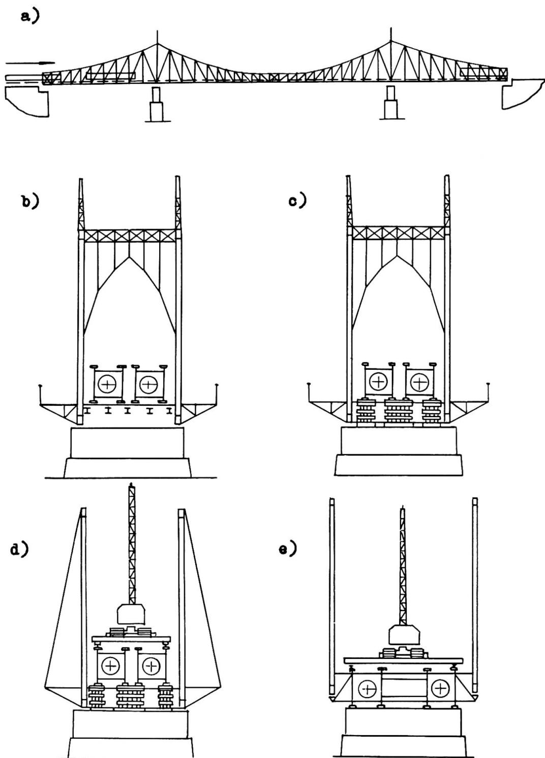
Fig. I The method of reconstruction of the metal superstructure of the Volga River Bridge in Kalinin: a, b- moving on blocks of the new superstructure; c- lowering of the moved on blocks onto the cades disposed on the permanent supports; d- cutting of lattice trusses into blocks and dismounting them; e- moving apart the blocks of the new superstructure and erection of lattice truss assemblies along the front of the new superstructure and their engaging.
