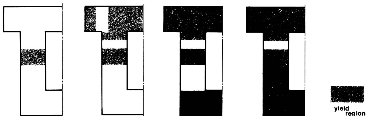
Fig.8 Progress of yield region in cross-section at every one hour (CC10).
