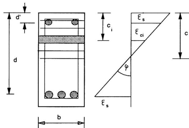
Fig. 2 Subdivision of compression zone in concrete layers
