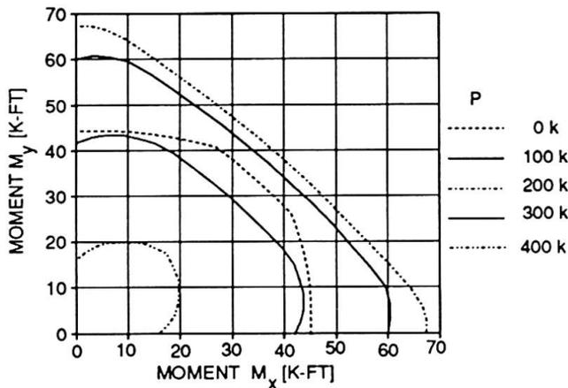
Finally, it is possible to let the neutral axis of the section rotate with respect to a fixed coordinate system which is parallel to the edges of the rectangular section. In this case one can obtain the interaction diagram for biaxial bending and axial load. Such a diagram is shown in Fig. 7. Each curve represents the ultimate strength of the section for combinations of bending moments  $M_x$  and  $M_y$  and a constant value of axial load  $P$ .
