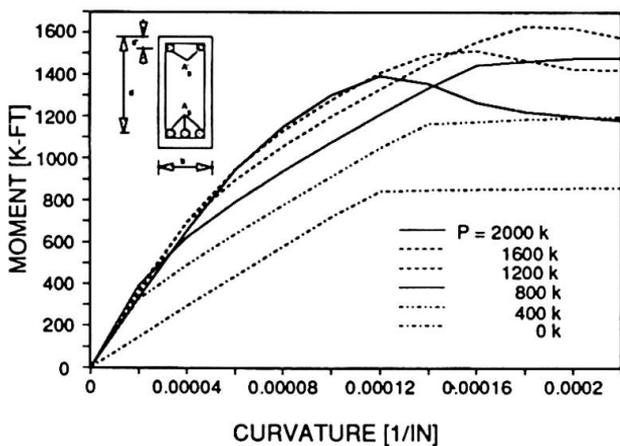
Fig. 5 Effect of axial load  $P$  on moment-curvature relation.  $\rho = 2\%, \rho' = 2\%, f'_c = 4$  ksi
