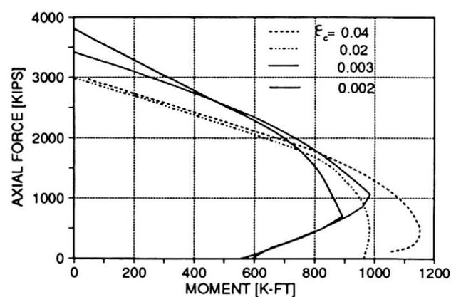
Fig. 6 Axial load-bending moment interaction diagram for a 20" square R/C column with  $\rho = \rho' = 2\%$  and transverse reinforcement of #4 bars at 2" o.c.,  $f'_c = 8$  ksi
