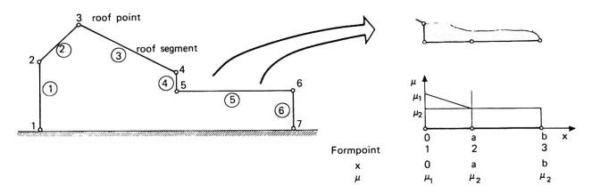
Fig. 2 Geometric model for roof profile and form function for roof segment
