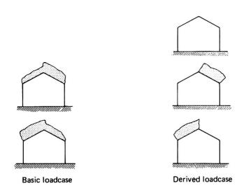
A derived load case represent a reduction of load on one or more segments or segment parts (Fig. 3). The concept of derived load case provides a mechanism for generating any number of load cases, as prescribed by NS 3479, cf section 3.2. This mechanism is, however, not included in the general numerical formulation.
