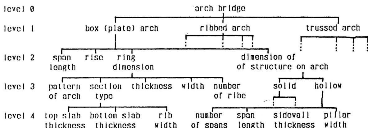
Fig. 4 Dimension data tree of arch bridge
