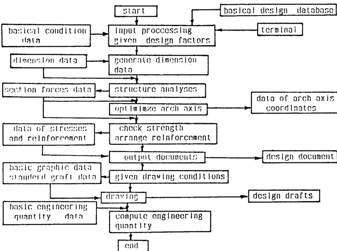
Fig. 3 Flow chart of data and modules
