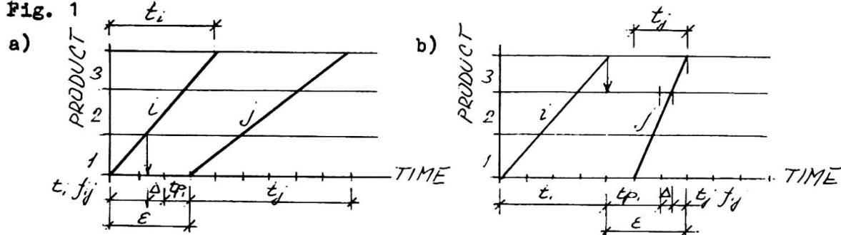
technology link can be converted to the finish-finish link and the lag time  $\epsilon$  can be calculated according to formula (2). The  $\Delta$  value rounds the lag time up so that the work gang  $j$  would start their work at a certain time unit in the morning.
