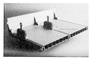
Fig.3 Model of the GRP enclosure floor for the Al9 Tees Viaduct
