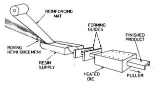
Fig.5 Diagram showing the pultrusion process
