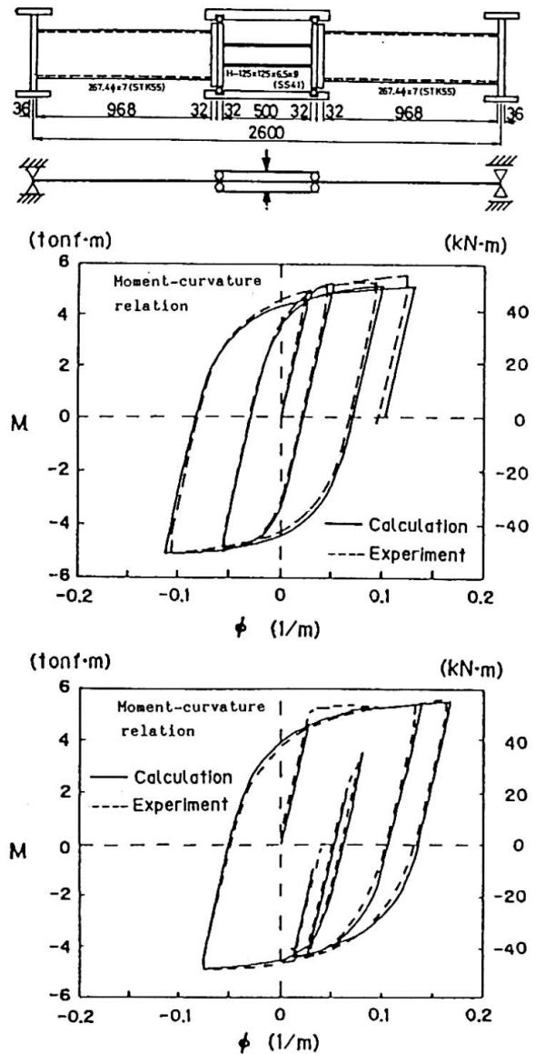
Figure 2 Moment-curvature relationships of simple beam specimens.
