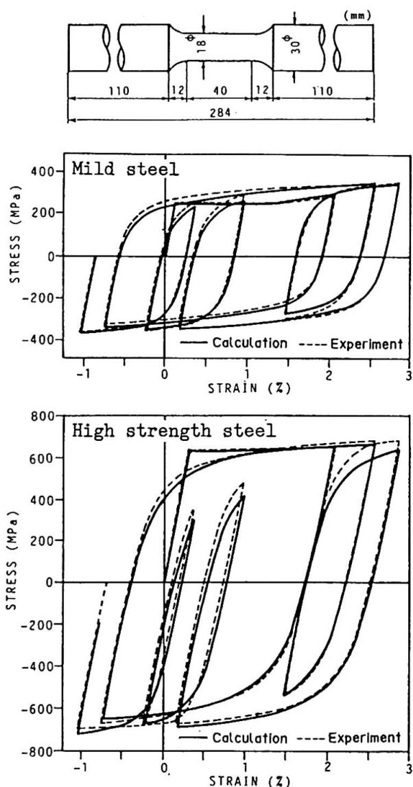
Figure 1 Stress-strain relationships of round bar specimens.
