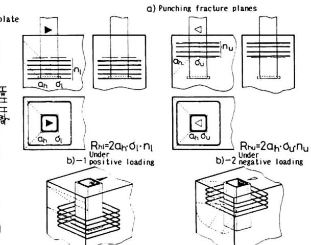
**Fig. 5 Assumption of three resistance conditions****Fig. 4 Assumption of punching fracture planes and working ties****REFERENCE**
